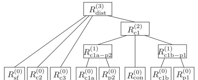
Fig. 6. Supervisor hierarchy of the distribution system.
